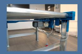
Motor under the conveyor Drive motor SEW placed under the conveyor.
