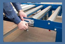
**Sensor mounting** Sensors and photocells can be mounted without any drilling and threading.
