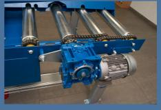
Motor on the side Direct drive on one of the rollers.
