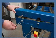
Service After loosen of two Height adjustment screws and removing the Hidden cover, there is a full access adjustment. for maintenance.
